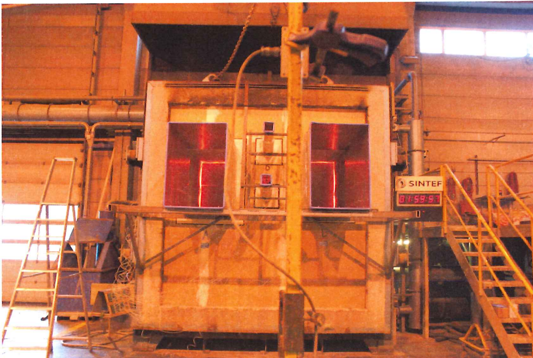
Photo 10: Unexposed face after 120 minutes. Note: ducts are glowing in the joint between the steel plates in bottom of duct.
