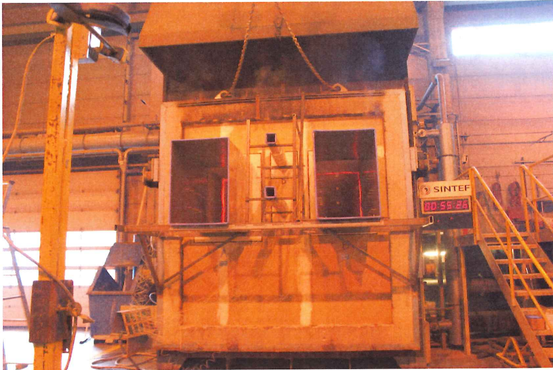
Photo 9: Unexposed face after 55 minutes.
